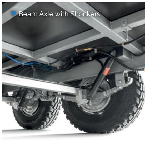
▼ Beam Axle with Shockers
